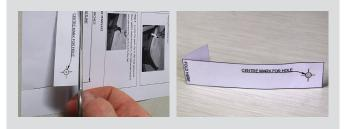
**Step 3:** Align the folded edge with the bottom lip of the cart making sure it is clear of any ribs or obstructions, then lay the template over the lid and mark the centre point keeping the template taut.
